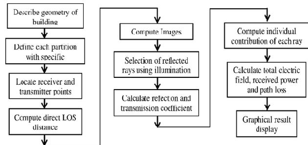
Figure 1: Flow Chart for Ray Tracing Model Implementation
