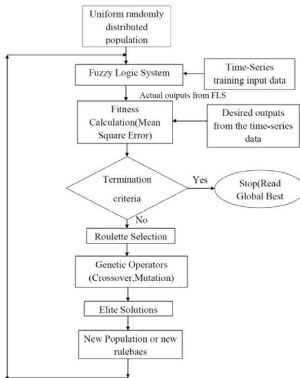
Fig. 4: Flowchart of Evolutionary Fuzzy Systems using Genetic Algorithm
