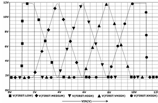
Figure 10(a). Transfer curves of *LOAD* Fuzzifier
