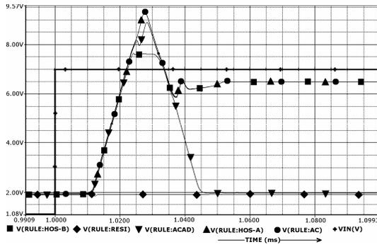
Figure 11. Time Delay after application of change at the input
