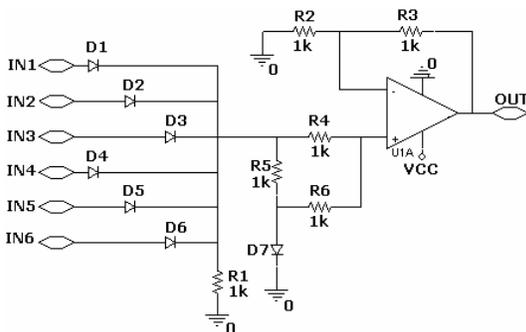
Figure 8. Fuzzy OR/MAX operator circuit
