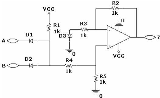
Figure 7. Fuzzy AND/MIN operator circuit
