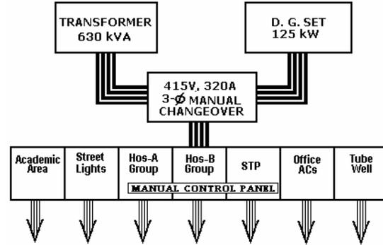
Figure 1. Layout of Power Distribution Control Room
