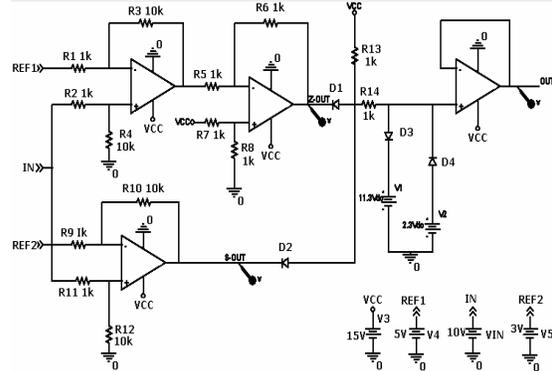
Figure 5. Tunable basic circuit for Triangular, Trapezoidal, S or Z-shaped membership function
