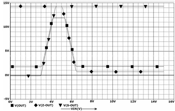
Figure 6. Simulated results for tunable circuit of Fig.5.
