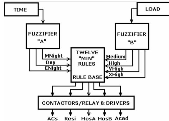
Figure 2. Block diagram of FLC for Automated Control Panel
