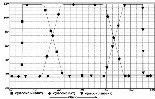
Fig. 10(b) Transfer curves of *TIME* Fuzzifier
